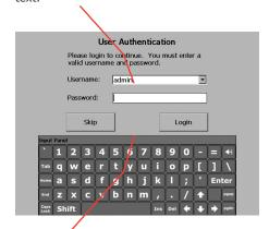
To move the onscreen keyboard to a new location on the screen, touch the stylus to the edge of the keyboard image and drag it to a new location.
